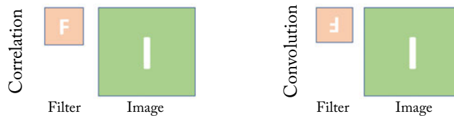
Figure 4.4: The distinction between the correlation and convolution operations in the signal processing literature. In machine learning, this distinction is usually not important and the deep learning literature normally refers to the layers implementing the correlation operation as the convolution operation. In this book, we also follow the same naming convention that is adopted in the machine learning literature.
