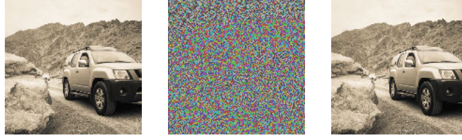
Figure 8.3: Illustration of the FGSM attack with \epsilon = 0.004 . Left: original image (classified correctly as a jeep). Middle: (magnified) adversarial noise. Right: perturbed image (misclassified as a minivan). Note that the added noise is substantially more perceptible for this attack than for the CW l_2 attack in Figure 8.2.
